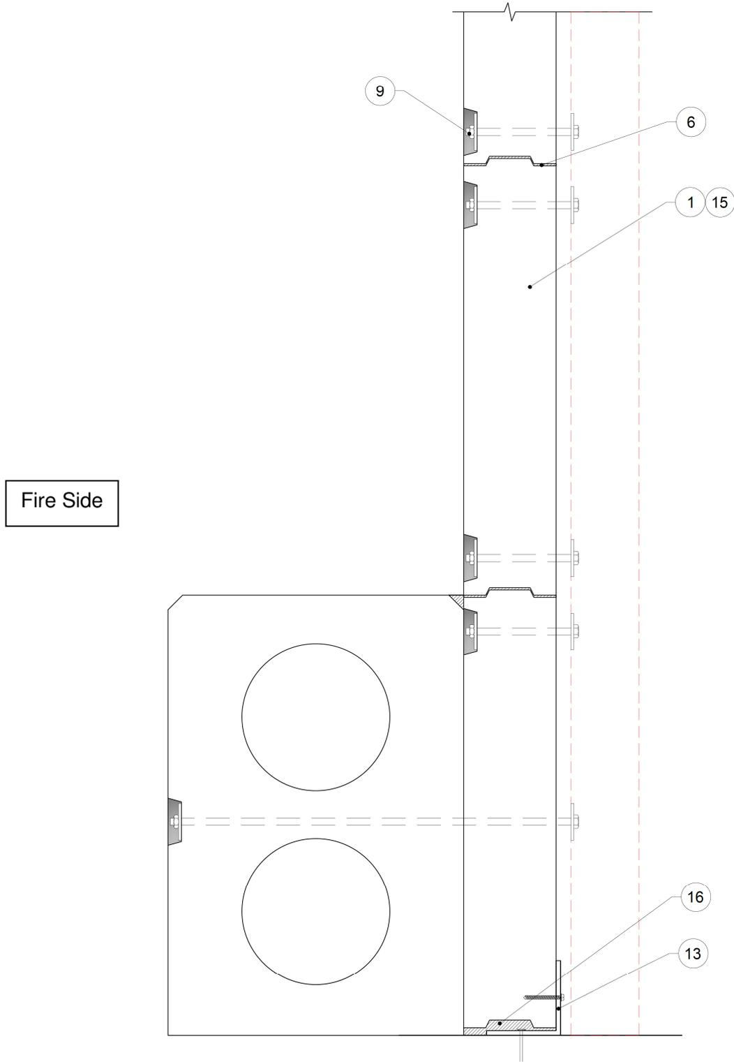
**Figure 11 – Service Panel Installation Option 2 (Tongue and Groove edge profile shown can optionally be nil profile for 150mm panels)**
