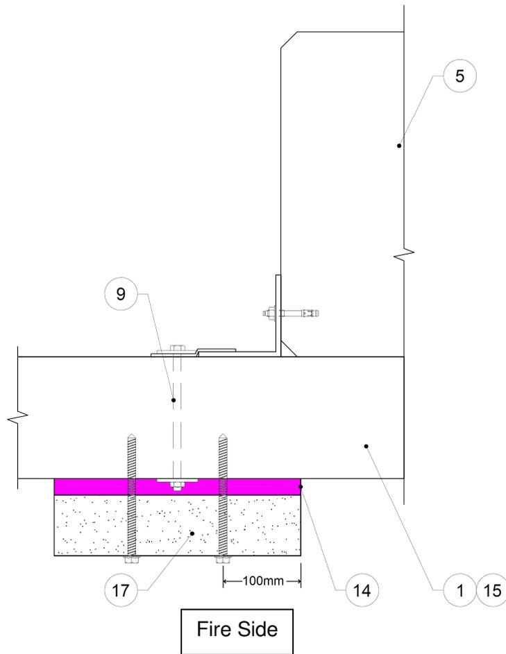
Figure 17 – Hebel Powerpanel or Powerpanel XL Bolt Shielding
