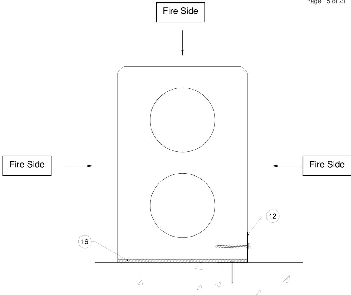
**Figure 13 – Service Panel Installation Option 4**
