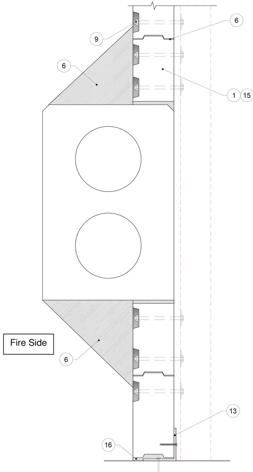
**Figure 10 – Service Panel Installation Option 1 (Tongue and Groove edge profile shown can optionally be nil profile for 150mm panels)**
