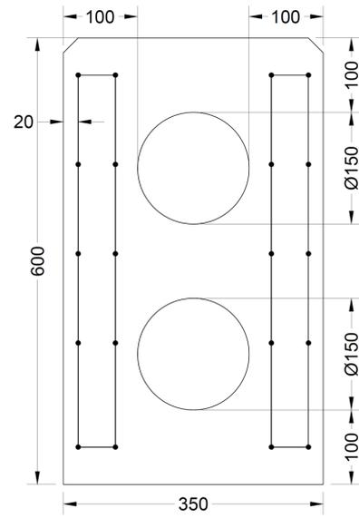
**Figure 9 – Hebel® Service Panel Type 2**
