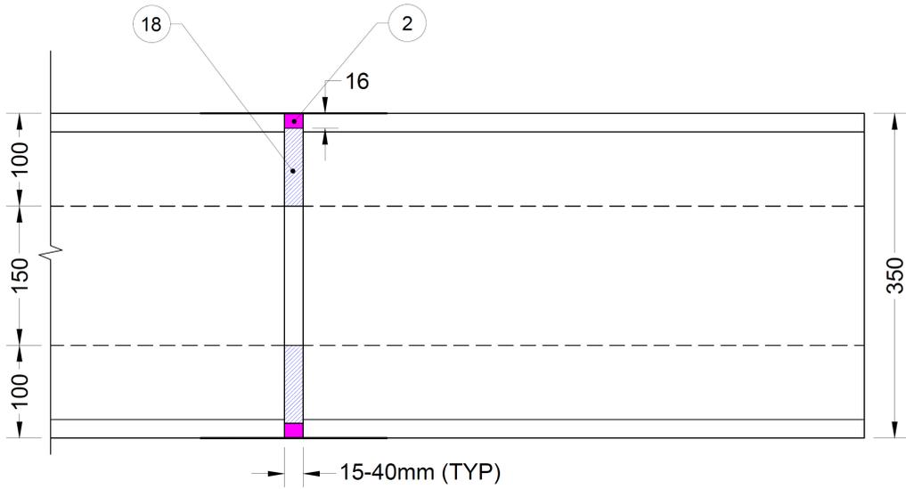
Figure 16 – Service Panel Type 2 Joint Detail –Plan View
