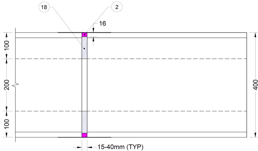
Figure 15 – Service Panel Type 1 Joint Detail –Plan View
