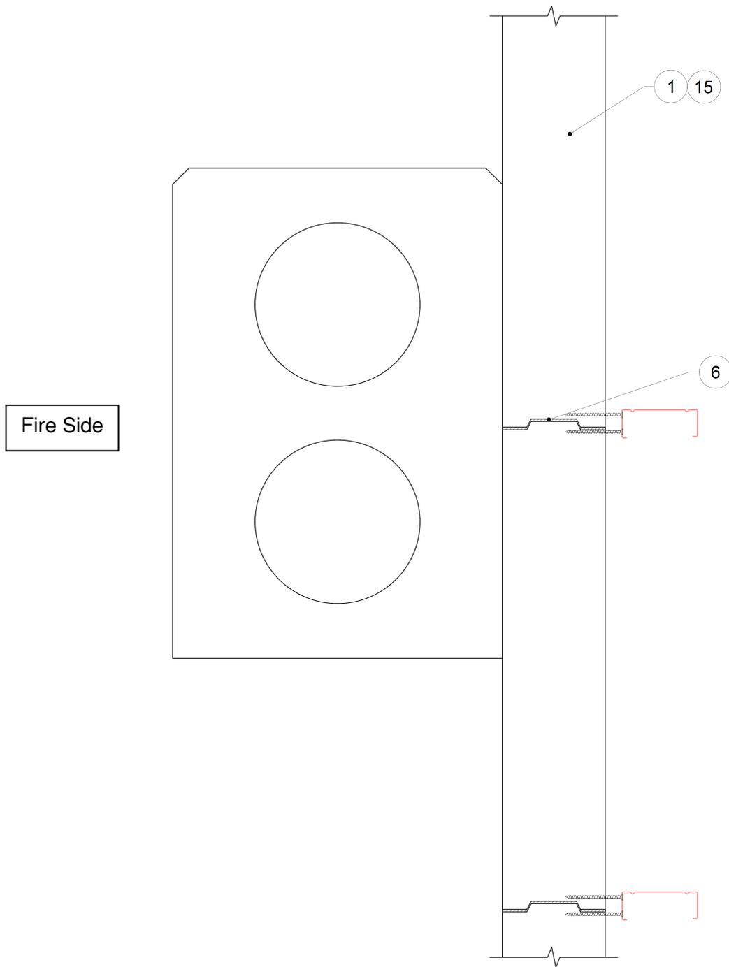
**Figure 12 – Service Panel Installation Option 3 (Plan View) (Tongue and Groove edge profile shown can optionally be nil profile for 150mm panels)**
