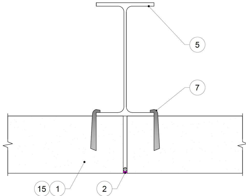
Figure 3 – Plan Section at Vertical Steel Column – Hebel Ties
