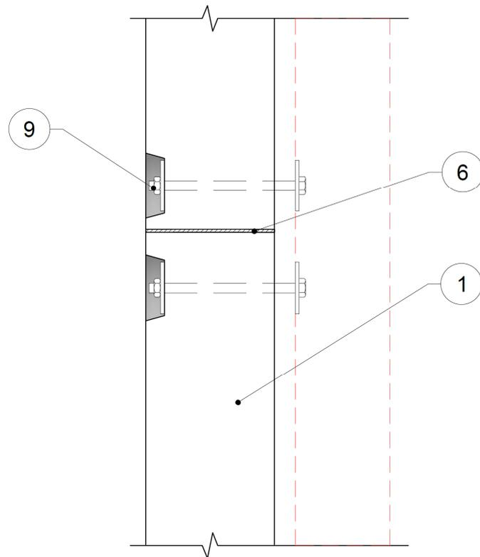
**Figure 18 – Example of nil profile edge of 150mm thick panel**
