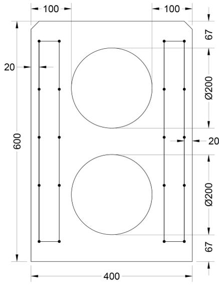
**Figure 8 – Hebel® Service Panel Type 1**
