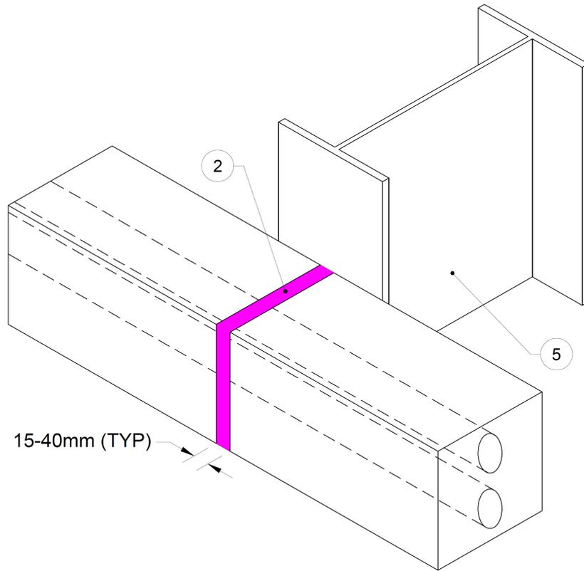
Figure 14 – Service Panel Joint Detail
