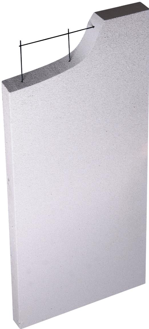
At the heart of the Hebel residential external wall system is the Hebel PowerPanel<sup>50</sup> - a 50mm thick, steel reinforced building panel made from AAC (Autoclaved Aerated Concrete) supplied in lengths of 2400mm with standard widths of 600mm.
